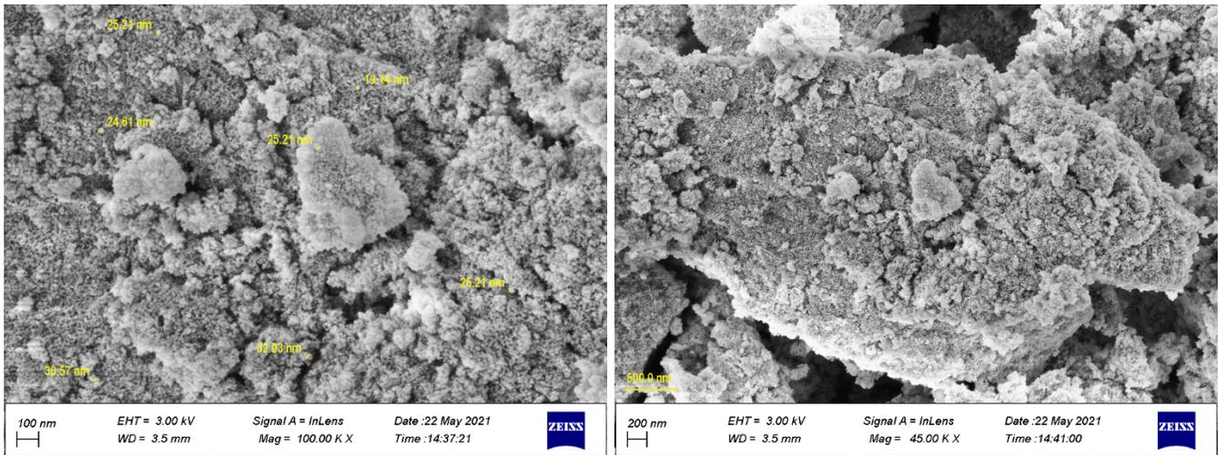
Figure 6. Scanning electron micrographs of CoO nanoparticles.
