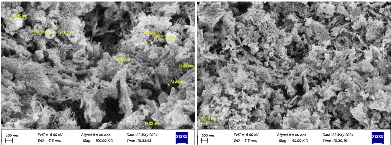
Figure 7. Scanning electron micrographs of ZnO nanoparticles.
