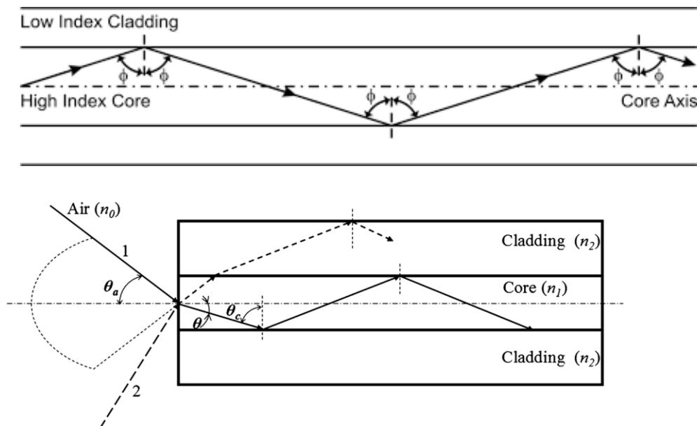
Light rays subtending an angle greater than critical angle will get guided by the fiber :
