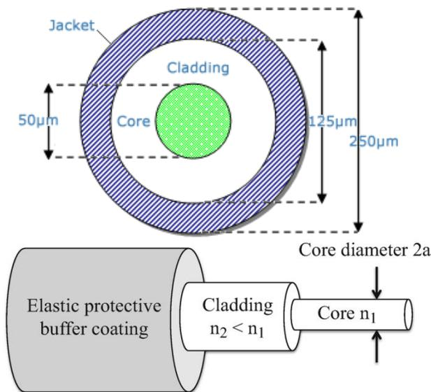
1. The optical fiber is a waveguide used for transmission of light. It consists of a dielectric fiber core, usually (pure silica), surrounded by a layer of (doped silica) characterized by the refraction index lower than that of the core, then coated by aluminum layer.
