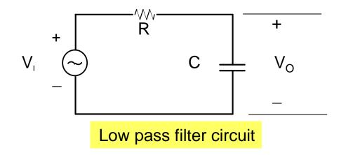
LPF: is a filter that pass low frequencies well, but attenuates or reduce frequencies higher than cut-off frequency.
