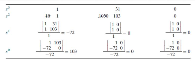
Because TWO changes in sign appear in the first column, we find that two roots of the characteristic equation lie in the right hand side of the s-plane. Hence the system is unstable.
