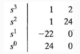
• Because TWO changes in sign appear in the first column, we find that two roots of the characteristic equation lie in the right hand side of the s-plane. Hence the system is unstable.
