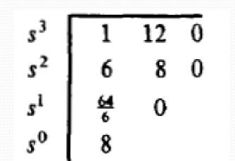
• Since there is no changes of the sign in the first column of the Routh table, it means that all the roots of the characteristic equation have negative real parts and hence this system is stable.
